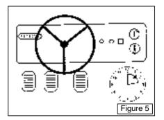
When the regeneration process is complete, only the green dash panel light and RPU power light will be illuminated.
