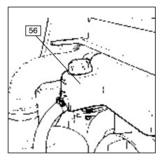
When replenishing, add a pre-mixed solution of water and anti-freeze of the same proportions as that already in the system.
