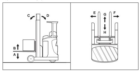
A / B Lowering/lifting the fork carriage C / D Tilting the lift mast (variant)
