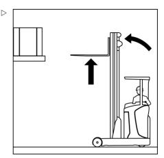
Extend the reach carriage until the fork back is resting on the load.
