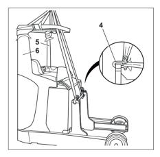
Hooking on the lifting straps to a truck without a lift mast
