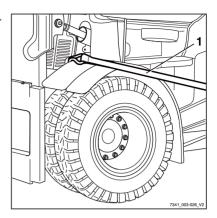
Attach lashing straps (1) to the coupling pin
