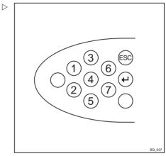
Keys for digits 0 to 9 for inputting the driver PIN  $\triangleright$  (access code)
