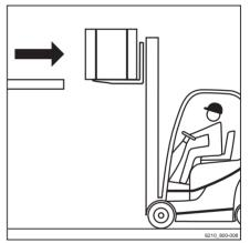
Lower the load while maintaining ground clearance.
