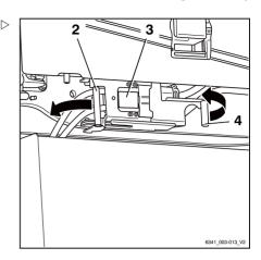
Hang the battery male connector (3) on the front edge of the battery tray (1).
