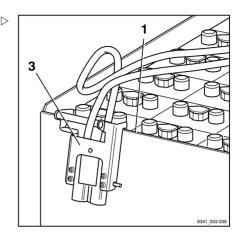
The slide rail (1) serves as an installation aid and guides the battery base frame at a right angle into the battery compartment.
