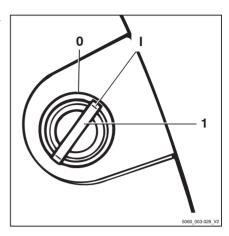
This initiates a self-test. All lamps in the drive direction and turn indicator displays light up briefly.
