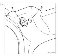
Switch the interior lighting (7) on or off using the switch (8) or button (1).
