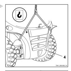
Adjust the length of the harnesses so that the lifting eye (6) is vertically above the truck's centre of gravity.
