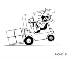
Do not overload the forklift. Check the load chart for load weight and load center information. Always pick up loads as close to the center of the weight as possible to avoid off-center loading.
