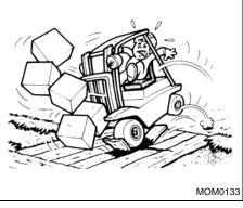
Avoid sudden starts, stops or turns. Slow down for turns and on uneven or slippery surfaces that could cause the forklift to overturn or slide.
