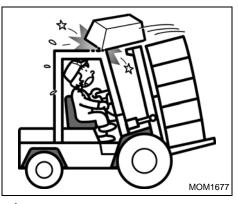
Do not place a load higher than the backrest of the forklift. A load placed higher than the backrest may drop towards the operator and is very dangerous. If such a load must be handled, securely fasten the load using suitable ropes or hold-down bands.
