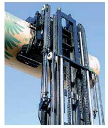
The free lift cylinders are equipped as standard with a hydraulic shock absorber to ensure elasticity and silence while lifting.
