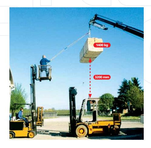
The MONTINI large capacity lift trucks undergo as well the impact testing of the overhead guards (also known as "Oregon Test").
