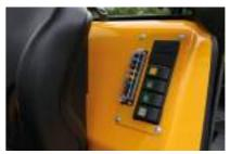
Electrical fuses can be easily checked and replaced.
