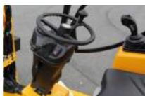
The steering column angle is adjustable. This is convenient and also makes getting in and out easier.
