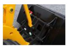
The "SWH" tool holder supports quick coupling and uncoupling of all equipment. Hydraulic locking is standard equipment.
