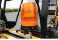
The optional rotating beacon is located in a protected position.
