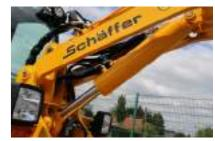
The lifting cylinder has been dimensioned to be particularly strong, thus matching the high tipping load. Swivel-head eyes protect against torsion.
