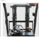
deliberate wide-view mast design focuses on the robustness and high interior quality to ensure safer operation and a wider
