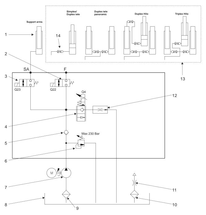
Pos. **Description** Pos. **Description** 1 Lift cylinder, support arm<sup>1</sup> 8 Tank Solenoid valve, fork selection [Q22] 2 9 Filter 3 Solenoid valve, support arm selection 10 Filter [Q23] 4 Proportional valve, lowering [Q4] 11 Air filter 5 Non-return valve 12 Flow regulator valve 6 Pressure limiting valve, max. 230 Bar 13 Lift cylinder, mast 7 14 Hose rupture valve Pump
