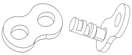
Wear to the bolts and around the holes on the discs is one reason why the chain stretches. The chain must be replaced if is stretched more than 2%.
