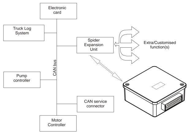
The picture above shows how the SEU is used to allow a greater number of functions to be controlled via the CAN bus. SEU has a 42-pin, multi-pin contact that manages all inputs, outputs, CAN and power supply signals.
