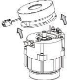
Remove the brake unit from the truck. Note the position of the brake so that refitting is done correctly.
