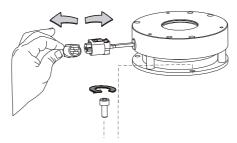
Remove the brake and the cable connector Q1.
