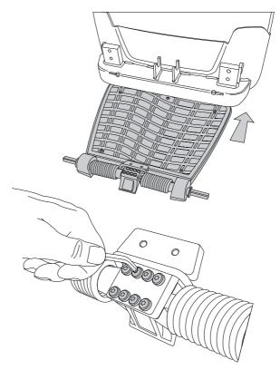
4. Loosen all 8 screws securing the bracket, which the spring clamp is pushing against.
