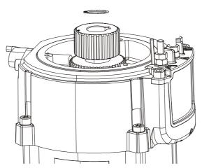
1. Remove the circlip
