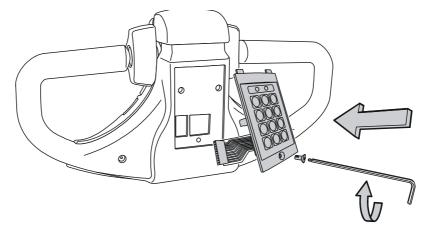
Connect the keypad and screw it in position
