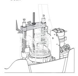
12. Unload the springs by prying up the bracket using the threaded bar.
