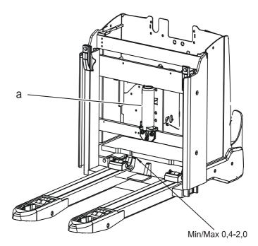
The gap between the chassis pressure plate and the support arm link roller must be between the minimum value of 0.4 and the maximum of 2.0.
