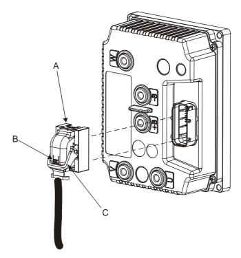
Keep the following in mind if it becomes necessary to disconnect the connector (A) of the transistor regulator:
