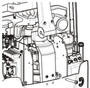
Remove the steering yoke from the truck together with the tiller arm (see the repair manual). Note the position of the conduit entry so that refitting is done correctly.
