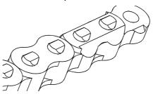
Maximal permitted outline wear is 5% of the thickness H2. If a lifting chain reaches the maximum level of wear, it must be replaced.
