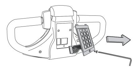
Detach the keypad and disconnect it from the logic card **Installing a keypad**
