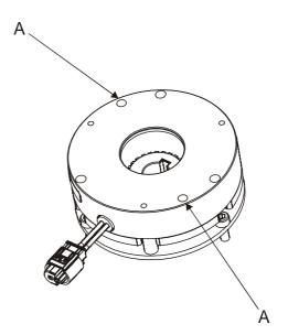
The brakes on the truck can be manually released by screwing two screws (M5) into the holes (A). The screws should be 30-35 mm long.
