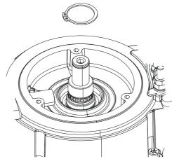
6. Remove the circlip from above
