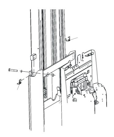
Tighten the screws that hold the mast
