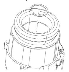
Remove the circlip inside the motor
