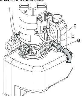
1. Pry off the sealing cap (a) attached to the pressure limiting valve using a screwdriver.
