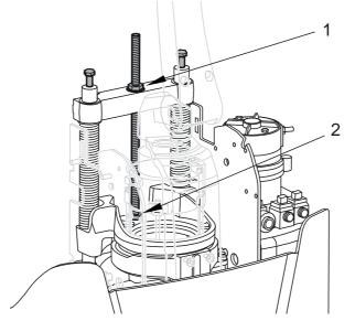
7. (1) Washer and nut on the top side. (2) Screw the shaft into the threaded hole and tighten with the nut.
