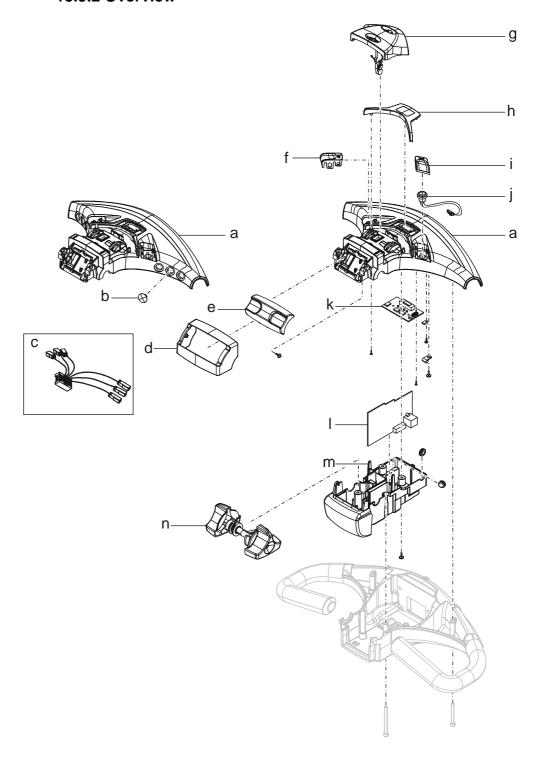
Description Pos. Cover а b Plug Wiring harness С d Cover Toggle switch е f Horn button Button "lifting/lowering" g h Display Horn button i Switch "horn" k Display 1 Electronic card "A5" Stomach button m Speed control n
