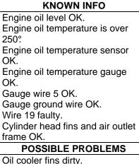
Oil cooler fins dirty Oil cooler faulty.
