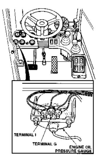
3. LOW ENGINE OIL PRESSURE (OIL PRESSURE GAUGE CONTINUOUSLY READS LESS THAN 30 TO 60 PSI [241-276 KPA]) (CONT).
