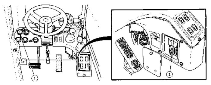
**a.** *Electrical System.* The forklift is equipped with a 24-volt electrical system. Status of the electrical system can be monitored by an ammeter gauge (1) located on the instrument panel inside the cab. A fuse panel (2) located under the instrument panel protects electrical circuits.
