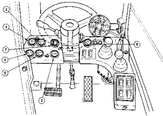
*f. Instruments.* All instruments are equipped with individual lamps for illumination and share a common circuit for power of these lamps. A common ground circuit is also shared for all instrument illumination. All instrumentation is fully operable when the main power switch and engine switch are on.
