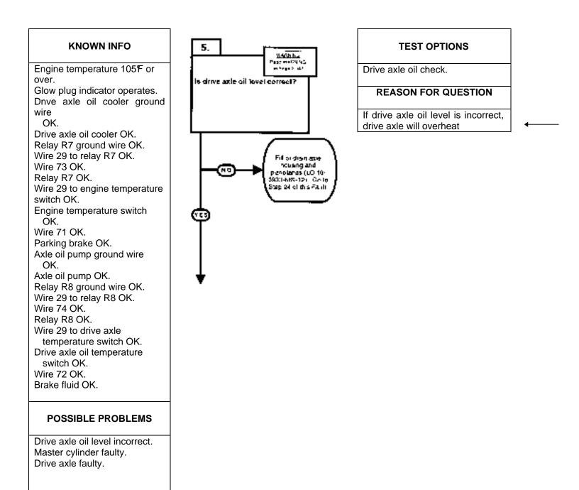
Drive axle and oil retains extreme heat. Do not check oil until drive axle has cooled. Failure to do so will result in severe bums to personnel.
