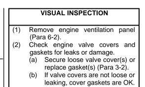
(3) Install engine ventilation panel.
