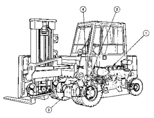
The forklift is powered by an air-cooled diesel engine (1) coupled directly to a semi-automatic transmission (2). Power from the transmission is transferred to the drive axle (3) through a short drive shaft (4) with two universal joints.
