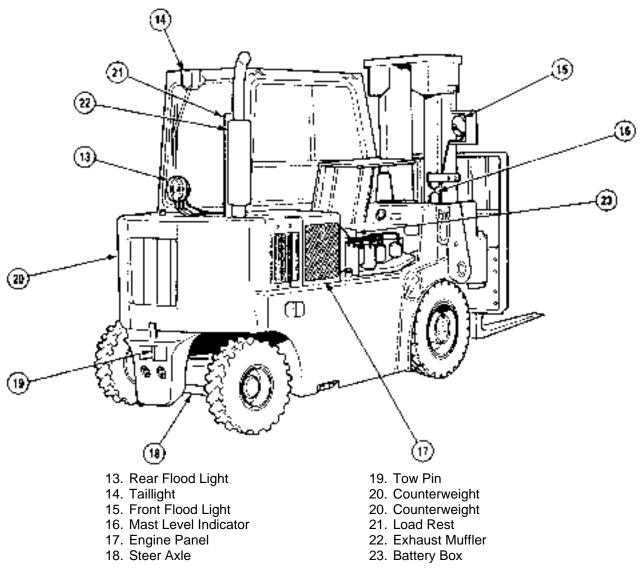
Figure 1-2. Truck, Lift, Fork - Right Rear View
