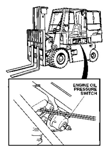
3. LOW ENGINE OIL PRESSURE (OIL PRESSURE GAUGE CONTINUOUSLY READS LESS THAN 30 TO 60 PSI [241-276 KPA]) (CONT).
