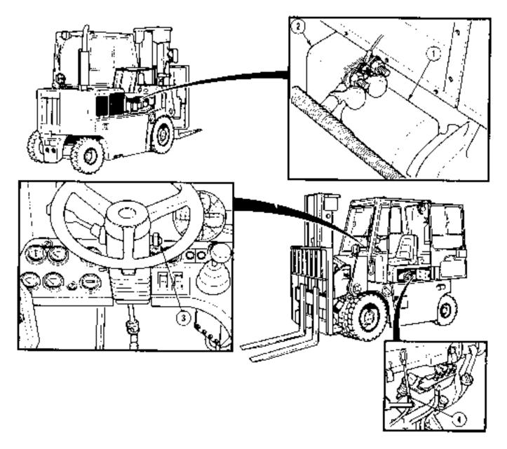
*d.* Engine Starting and Stopping. The engine starting system consists of a starter motor (1), solenoid (2), and engine switch (3). Battery voltage is used to operate the starter motor (1). The starter motor (1) is mounted on the engine and engages the flywheel only when electrically energized. When the engine switch (3) is turned to the OFF position, the fuel shutoff solenoid (4) is de-energized causing the injection pump to stop fuel supply to the injectors.
