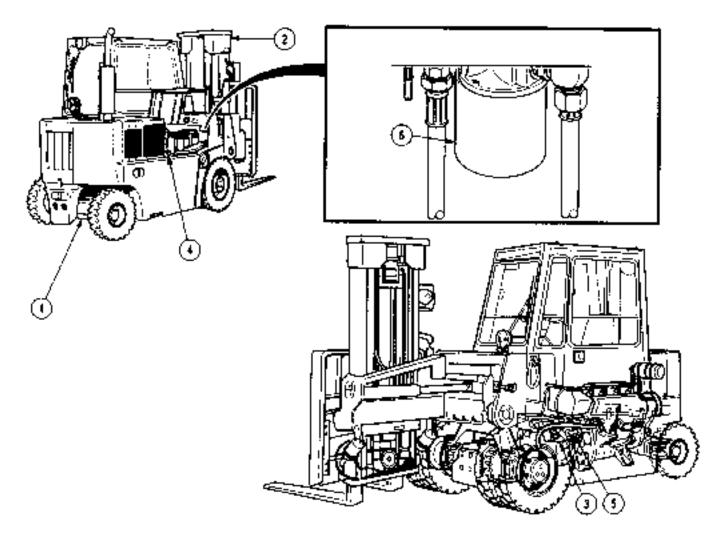
The hydraulic system supplies hydraulic oil pressure for steering (1) and mast (2) operation any time the engine is running. A pump (3) mounted on the transmission draws hydraulic fluid from the hydraulic tank (4) mounted on the RH side of the forklift. A priority valve (5) diverts hydraulic fluid to the mast (2) and steering (1) system by demand. Hydraulic fluid is filtered by a spin-on filter (6) immediately before returning to the hydraulic tank (4).
