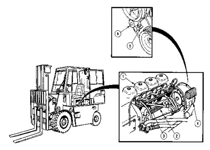
**a.** Cooling System. The cooling system protects the engine (1) from excess operating temperatures by removing heat generated during the combustion process. Air is drawn through the engine oil-to-air cooler (2) and then past the engine cooling fins (3) by a belt-driven blower (4). A sensor (5) is located on the blower belt tensioner (6). This sensor will send voltage to a warning buzzer and a warning light on the instrument panel when the blower belt breaks or comes off its pulleys.
