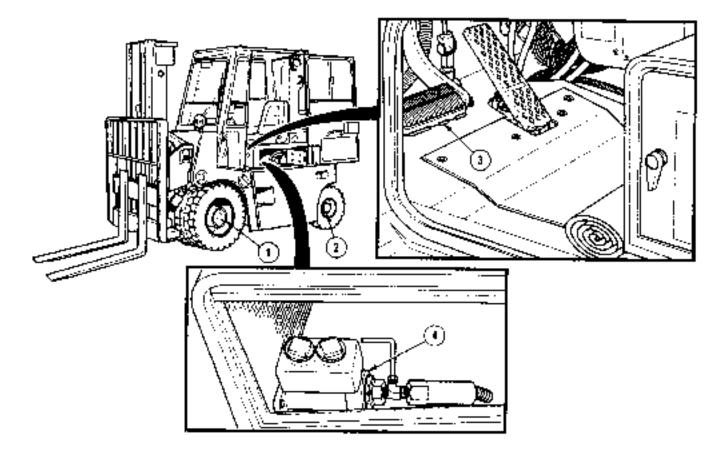
The forklift brakes are located inside the drive axle (1). The steering axle (2) is not equipped with brakes. Braking is controlled by the brake pedal (3) which is connected to the master cylinder (4) by a linkage. Additionally, the brake pedal (3) disengages the transmission automatically as the brakes are being applied.
