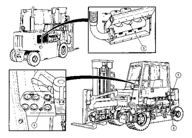
**b.** Air Intake System. The air intake system consists of a dry-type filter contained in an air cleaner (1), ducting (2), and the engine intake manifold (3). Condition of the air filter is monitored using the air filter indicator (4).
