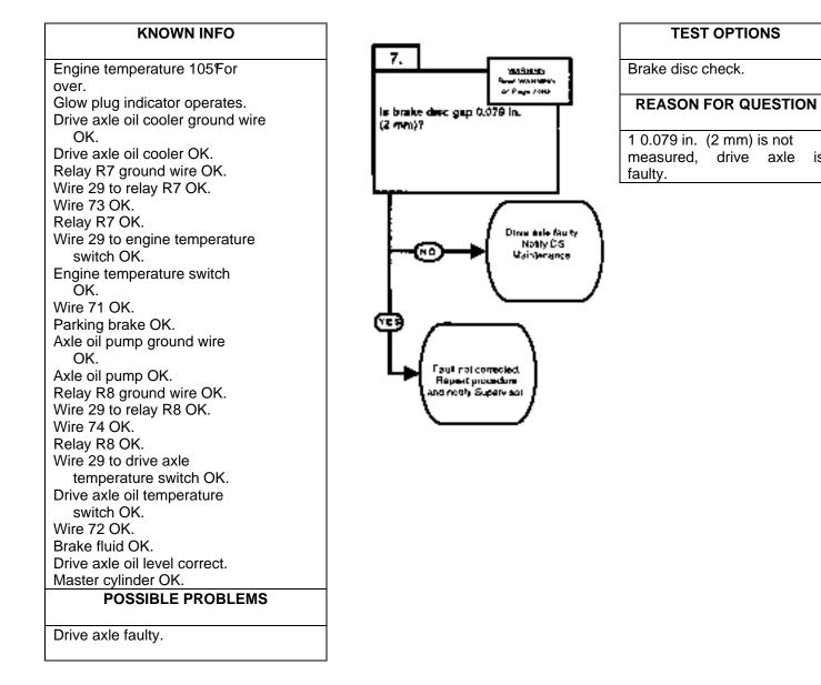
Drive axle and oil retains extreme heat. Do not check oil until drive axle has cooled. Failure to do so will result in severe bums to personnel.
