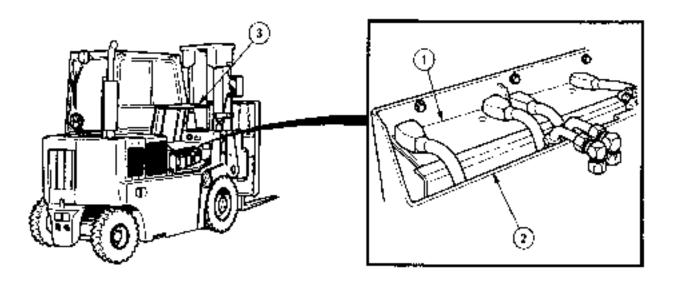
**b.** Battery. The electrical system is equipped with two 12-volt batteries (1). The batteries are contained in a battery box (2) located on the right-hand side of the forklift under the engine access cover (3). This location provides protection from the environment while allowing convenient access for service.
