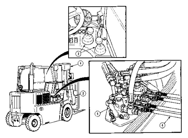
All functions of the mast assembly (1) and the pivot/shift assembly (2) are controlled by two joysticks (3) mounted in the cab. Joysticks (3) are connected by cables (4) to the stack valves (5) which direct flow to and from the mast assembly (1) and pivot/shift assembly (2). Hydraulic oil pressure is provided by a transmission-mounted pump which is shared by the steering system, mast assembly, and pivot/shift assembly.
