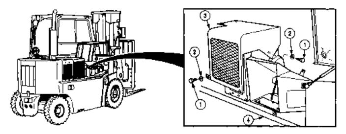
(1) Remove five screws (1), washers (2), and ventilation panel (3) from forklift (4).
