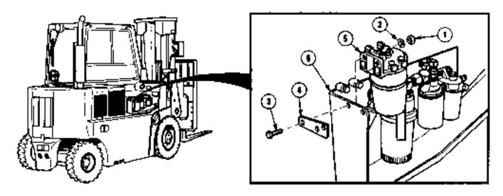
(1) Remove two nuts (1), washers (2), screws (3), bracket (4), and fuel/water separator (5) from filter tray (6). Position fuel/water separator clear of filter tray.
