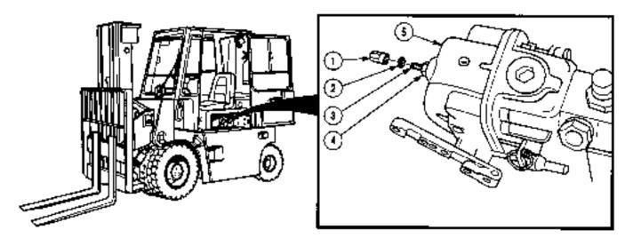
Remove nut (1) and seal (2) from idle adjustment screw (3) and locking nut (4) on governor (5). Discard seal.
