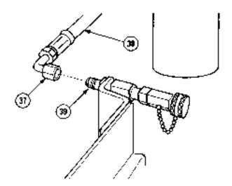
(2) Install hose (38) on AOAP valve (39) and tighten fitting (37).
