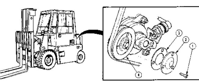
(1) Remove three screws (1), cover (2), and gasket (3) from blower belt tensioner pulley (4). Discard gasket.
