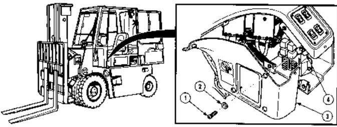
(1) Remove seven screws (1), washers (2), and lower dash panel (3) from dash frame (4).
