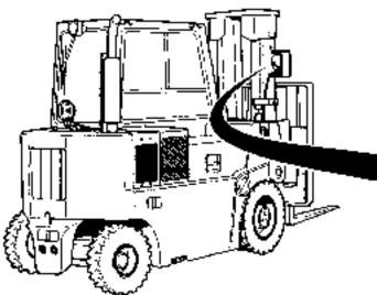
(1) Disconnect connector (1) from light connector (2).
