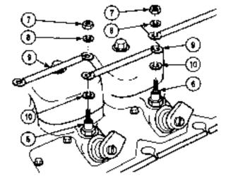
(4) Install washer (5), two wires (4), washer (3), lock washer (2), and nut (1) on glow plug (6).
