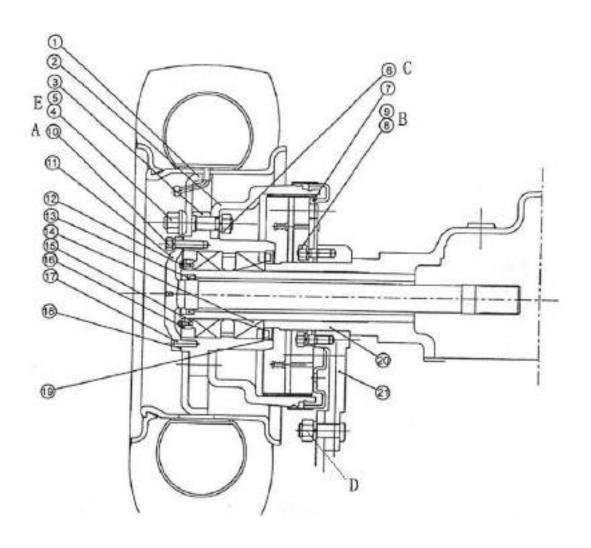
Fig.3-1 Driving axle
