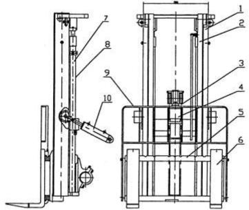
Fig5-2 Double full free lift mast
