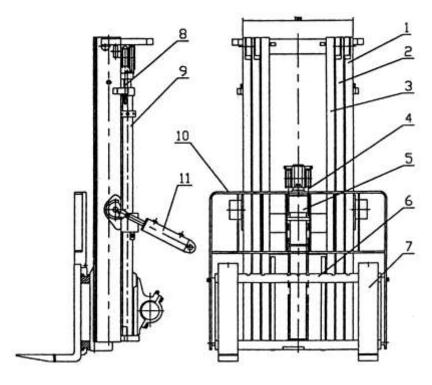
Fig 5-3 Container truck mast
