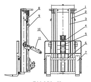
Fig 5-4 Triple full free lift mast
