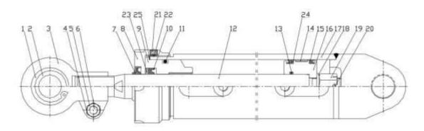
Fig 5-6 Tilting cylinder
