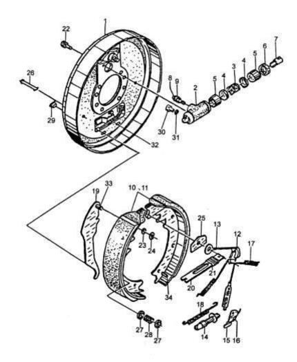
Fig.3-2 2-3t forklift truck right brake assembly
