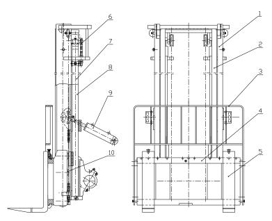
Fig5-1 Double lift mast with wide view
