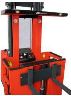
Halogen spots in the overhead guard and a fork carriage with adjustable forks are standard.. The ergonomic control panel with handle bar for safe operation.
