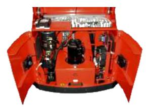
With the AC-Drive motor high acceleration and speeds are possible.
