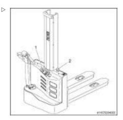
Turn the key switch (1) to the ON position; the battery indicator light will come on.
